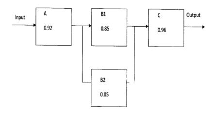
$$\begin{split} R_{bb}{}^{1} &= Q_{bb}{}^{1} \\ Q_{bb}{}^{1} &= (1\text{-}0.85) \ (1\text{-}0.85) = 0.0225 \\ R_{bb}{}^{1} \ 1\text{-}0.0225 = 0.9775 \\ R_{B} &= 0.92 x 0.9775 x 0.96 \text{=} 0.86 \end{split}$$
